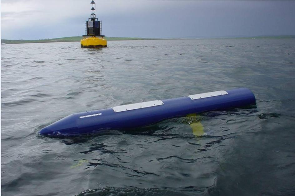
*View of a 1/20<sup>th</sup> scale prototype tidal generator device*
