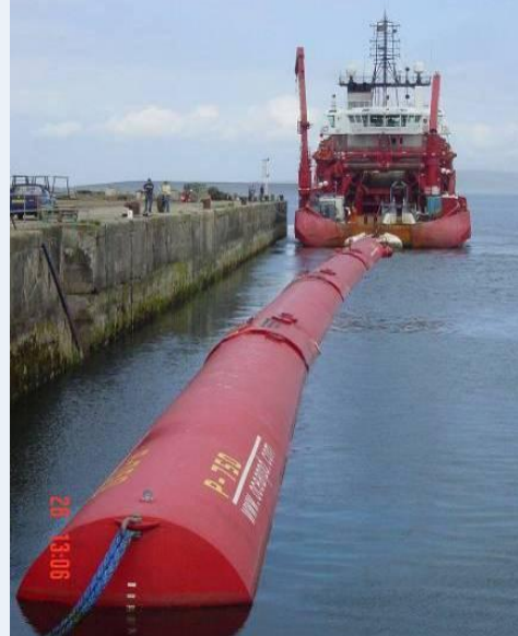
Pelamis awaiting deployment in Orkney
